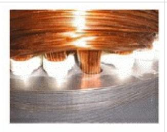
This picture shows a slot in which the slot insulation is missing. The winding wire touches the lamination or is a small distance away from it.
