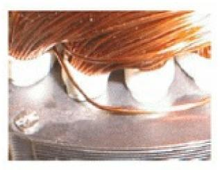
The picture shows a loose winding wire. The winding wire touches the lamination or is a small distance away from it.
