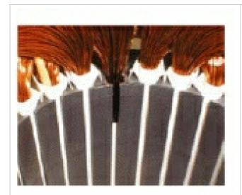
The picture shows a slot in which a part of the slot liner is missing. The winding wire touches the lamination or is a small distance away from it.
