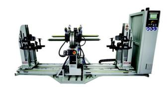
The coil forming process is achieved through movements generated by the pneumatic cylinders. The movements can be performed either individually to allow a quick and easy changeover or sequentially and automatically.
