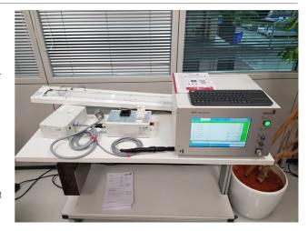
Continuity test and polarity check for luminaries with power connections through the lamp
