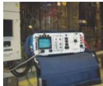
Shown here is the Baker AWA, Automatic Winding Tester, in use with Microgen Energy Ltd, a subsidiary of BG Group.
