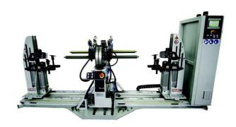
2 clamps for the stator slot length are provided. These clamps are used to hold and shape the radii of the coil during the opening phase. They are manually positioned according to the required lengths. The clamps are designed for a quick set up when changing the batch.
