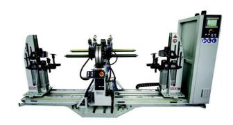
The coil forming process is achieved through movements generated by the pneumatic cylinders. The movements can be performed either individually to allow a quick and easy changeover or sequentially and automatically.
