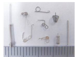
Torsion spring parts formed on SH-311
