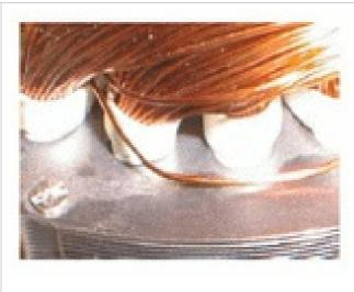
The picture shows a loose winding wire. The winding wire touches the lamination or is a small distance away from it. In a high-voltage test such a defect is only detected with either a very high test voltage (not always possible) or if the winding wire is
