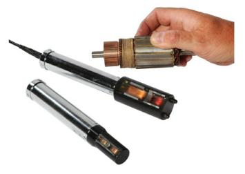
Growlers will work on any armature where the coil can be isolated magnetically. Typically these are found in DC armatures, though some AC rotors, depending on how they are wound, may also be tested. In an AC motor, if there is a squirrel cage or other type of ring that prevents individual coils from being isolated magnetically, then this may interfere with a growler's ability to function"
