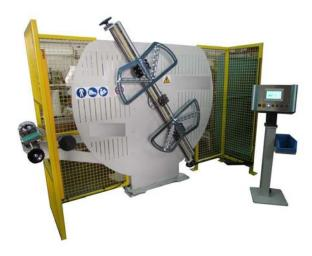
The most versatile, operator friendly and cost effective solution for coil or pole winding applications. MX machines have been specifically designed and built for the quick and precise winding of copper bars or wire up to 3000 mm (max reel length).
