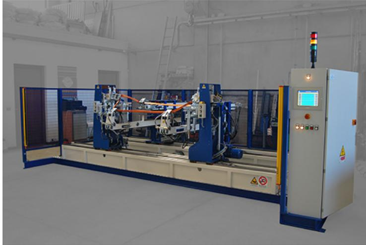
***Highly versatile machine specifically built for the automatic forming of a wide range of coils, with maximum length up to 3500 mm. Thanks to its hydraulic cylinders, this machine proves to be highly powerful and suitable for the mass production of various kinds of big-size coils.***
