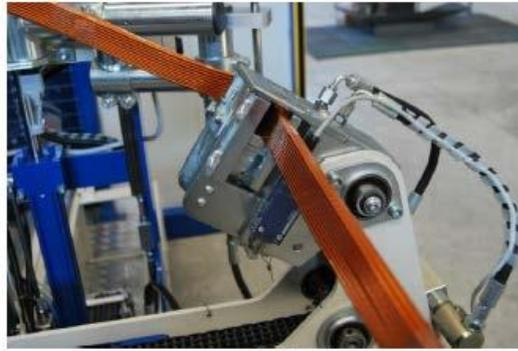
Equipped with hydraulic cylinders for retaining the copper bar with the possibility of varying the locking position depending on the section of the coil that has to be formed.
