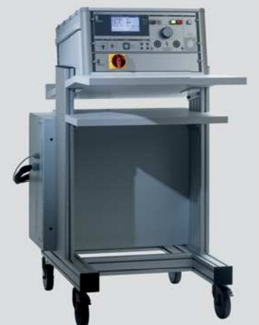
GLP2 with 6KV/1A on a rolling table and safety door
