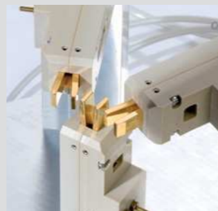
Contacting of contact pins with Kelvin clamps
