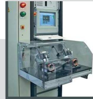
Dual station with MTC3 in 19"-cabinet
