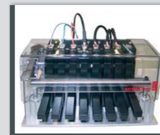
Block with Kelvin clamps with automatic release
