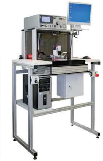
Single test cage and work table with deposit tables at the sides and GLP2
