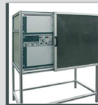
High-voltage test station up to 40KV
