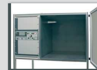
GLP2 with test cage for 40KV AC and safety door
