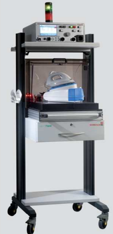
Rolling table with integrated test cover, drawer element and cable holders
